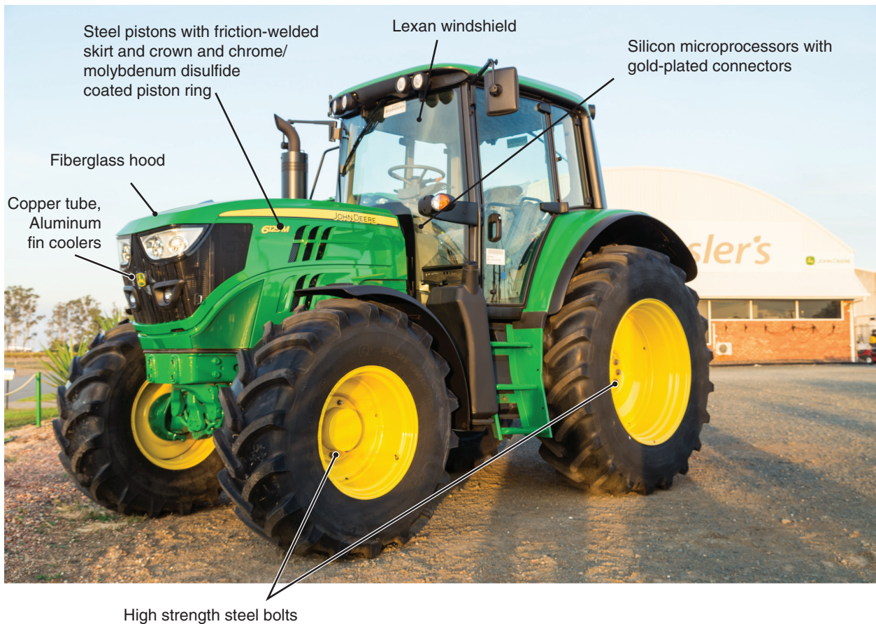
Figure I.2: John Deere tractor showing the variety of materials and processes incorporated. Source: Shutterstock/Nils Versemann.
